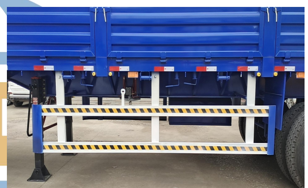
Heavy loading 19 Inch Two speed landing gear Strong Side fence to protect the trailer
